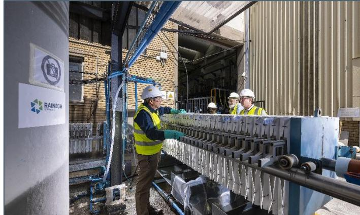
Filter press at the front-end pilot plant
