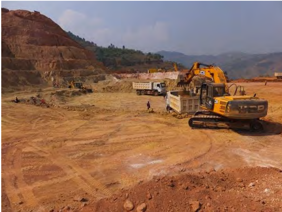
Plate 15: Showing bulk waste mining and selective mechanical mineralised material mining
