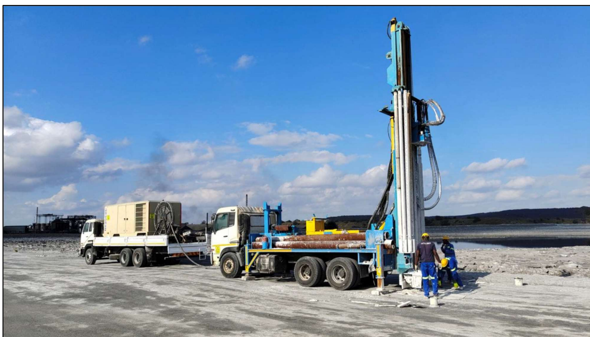
Figure 8.3 Open-hole RAB drill rig
