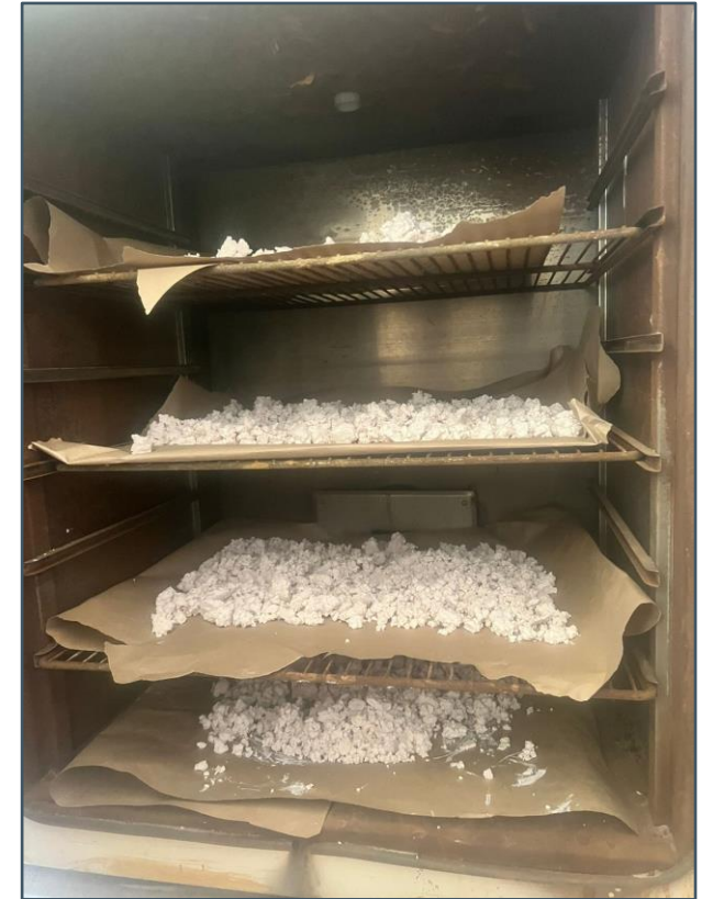
Initial production of mixed rare earth sulphate above
