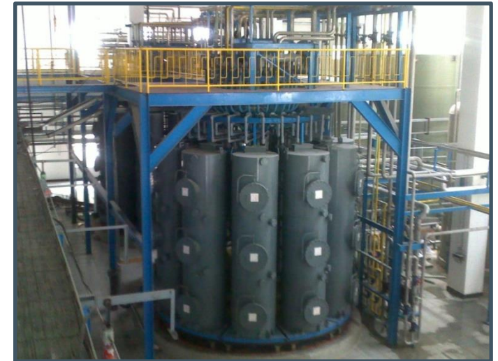
An example of a commercial scale CIX unit built by K-Tech
