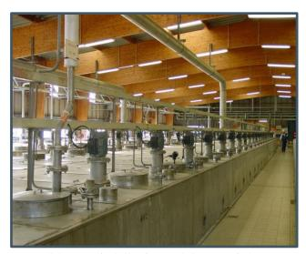
Rare Earth SX separation battery in La Rochelle, France; just one small fraction of overall process
