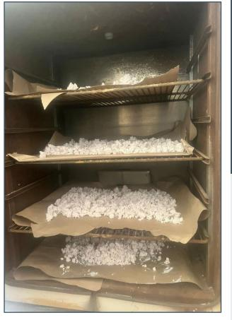
Mixed rare earth carbonate successfully produced by front-end pilot plant
